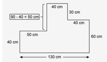
(b) Total surface area = 2 x Area of cross section+ Area of bottom face+Area of left face+ Area of right face+Area of top face
